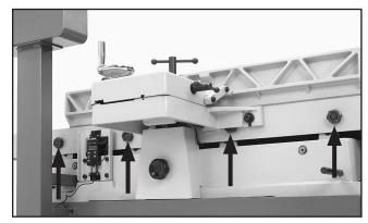
Figure 53. Rear eccentric bushings.
